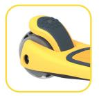
**Safety First** The Glider Air features a wide foot brake, allowing for easier stopping and control.
